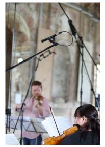
distinct suppression of sound signals coming from the side, the MKH 30 ensures very good acoustic separation of individual instruments when used as a spot mike, thus allowing interfering room modes that run perpendicular to the main axis of the microphone to be effectively cancelled out.
