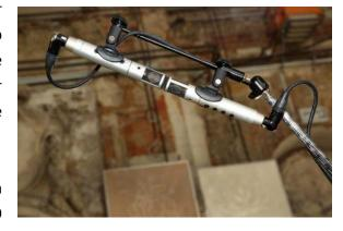
degrees to one another (figure-of-eight). One microphone was pointed directly at the instrument while the other may possibly be used in the mixing process as a signal supplier for an M-S matrix. According to Jakob Händel, the double figure-of-eight provided pleasant "bite".
